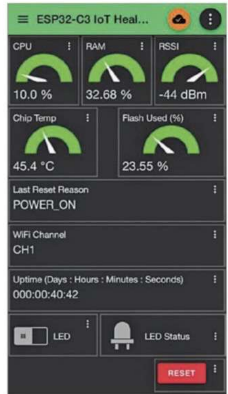
Fig. 18: IoT MQTT Panel dashboard displaying real-time ESP32-C3 Super Mini telemetry, onboard LED control, LED status, and remote reset functionality
